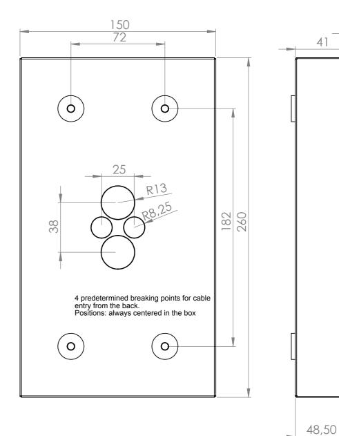
Predetermined breaking point at the bottom All breakouts for cable entry are closed and designed as predetermined breaking points.
