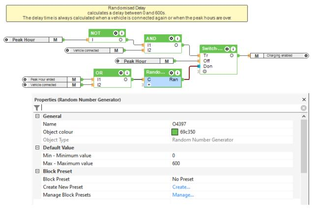
If a vehicle is connected and you are outside the peak hours, a random number between 0 and 600 is generated. As per the regulations, this can be remotely increased to up to 1800 seconds if required provided the option for remote configuration of that Miniserver has been completed. After this time has elapsed, charging permission is only given for the corresponding charging station.
