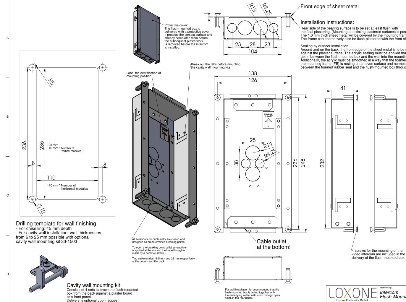
Rear side of the bearing surface is to be set at least flush with the final plastering. (Mounting on existing plastered surfaces is possible). The 1.0 mm thick sheet metal will be covered by the mounting frame (FB). The frame can alternatively also be flush-plastered with the front of the sheet metal.
