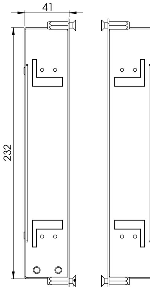
4 screws for the mounting of the video intercom are included in the delivery of the flush-mounted box.
