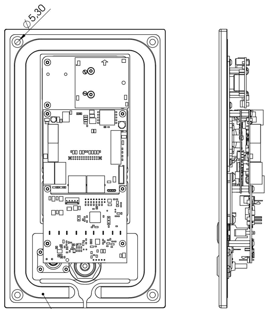
Sealing with foam rubber tape 10mm
