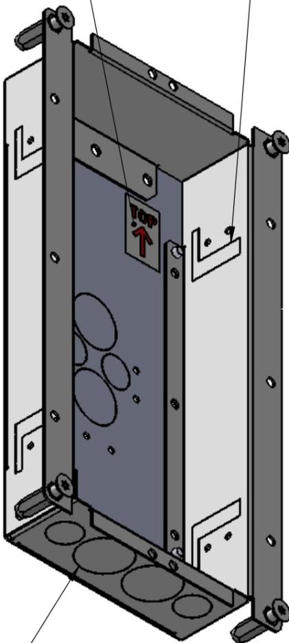
Break out the tabs before mounting the cavity wall mounting kits
